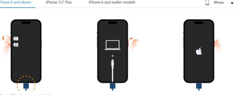
1. Power off the device, connect it to the computer via a data cable. Press the volume up button once, then press the volume down button once
