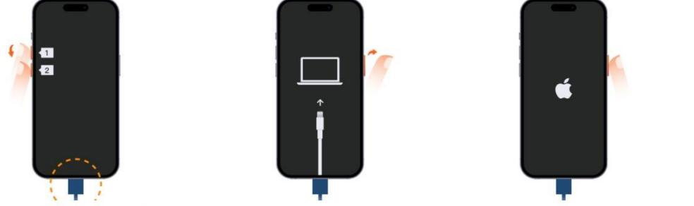
1. Power off the device, connect it to the computer via a data cable. Press the volume up button once, then press the volume down button once
